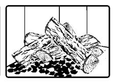
Remove ash first, and then rake charcoal towards the front of the firebox before loading so that it will ignite the new load.
