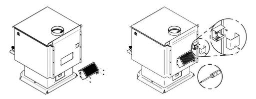
The blower has a rheostat, see the illustration on the right to identify the different adjustment positions; either from high (HI) to low (LO) or turned off (OFF).
