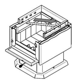
1- Starting with the rear tube, lean and insert the right end of the secondary air tube into the rear right channel hole. Then lift and insert the left end of the tube into the rear left channel.
