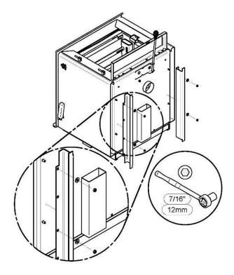
3- Remove the (2) transport support bracket which can be discarded. Keep the (4) bolts, washers and nuts since they will be required in **step 5**.
