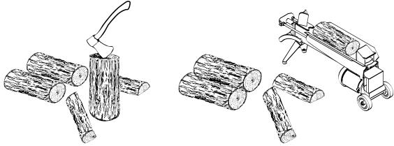
Wood should be split to a range of sizes, from about 3" to 6" (75 mm to 150 mm) in cross section. Having a range of sizes makes starting and rekindling fires much easier. Often, the firewood purchased from commercial suppliers is not split finely enough for convenient stoking. It is sometimes advisable to resplit the wood before stacking to dry.
