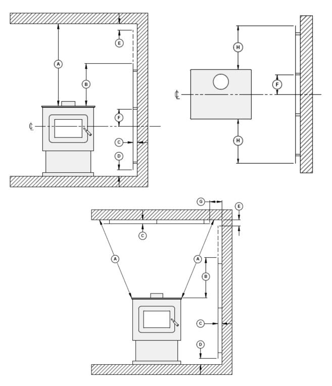
**Clearances for shield construction**
