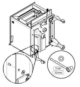
5- Secure both leg support assembly to the underside of the firebox using the bolts, washers and nuts removed in **step 3**. Supports can be installed on either side.
